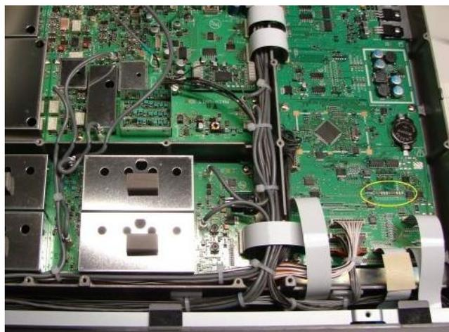
This reveals the section where jumper pins are located that control the processor where a jumper is required across position 04.
