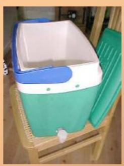
The *MASH TUN* is a made from a converted cool-box. The polystyrene insulation has been 'beefed up' with an inner and outer layer of aluminium foil, shiny side in. This improves its ability to retain heat, vital for a good *predictable mash*.
