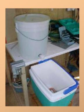
The *Hot Liquor Tun* is shown here with 20 litres of 'liquor' (treated and heated water) ready for running into the mash tun. Gravity saves a lot of messing about! Victorian brewhouses were often 'gravity assisted' (Tower Breweries).
