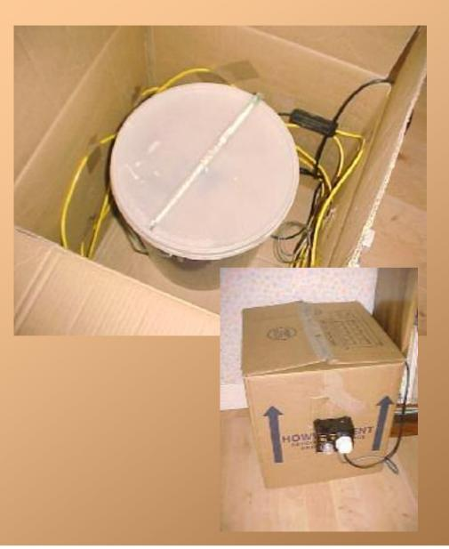
To ensure a reliable *fermentation* in winter, a heated box is used controlled by a thermostat.
