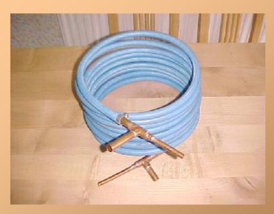
An alternative to the *crash* cooling coil is the counter flow cooler, where hot wort goes one way and cold water goes the other way.
