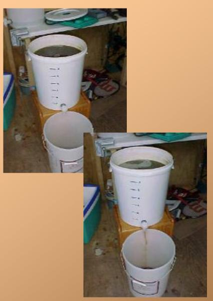
Once cooled to 25 degrees centigrade the wort is run off into the fermenting vessel. The height drop is deliberate as to propagate and perform its task yeast needs oxygen. Aeration is avoided during the early stages of brewing as oxidation of the hot wort is undesirable - it can produce 'off' flavours.
