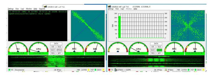
Normally, you setup 2 x monitor screens – the one on the left is the normal receive monitor and shows incoming text and the decode data. The one on the right is monitoring my connection and shows many items of information including the data rate (in this case approx. 270bps which is over double the speed you can reach on the "freebie" version).
