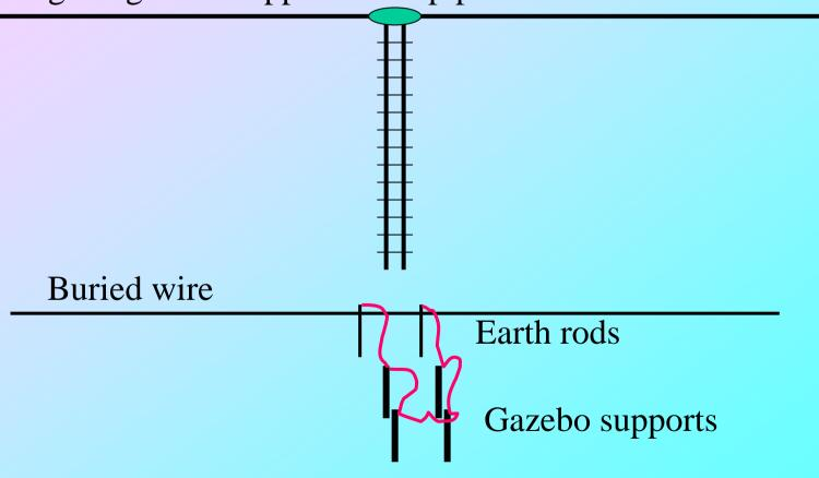
The gazebo supports were interconnected using more 2.5mm<sup>2</sup> and plenty of grease to prevent corrosion. Placed several years ago, steel pipe doesn't decay quite as quickly as wood!
