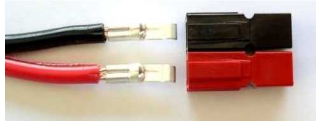
Picture above of correctly crimped Anderson PowerPoles
