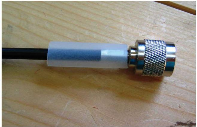
I usually add some heat shrink sleeving to give some added protection to the crimp sleeve. In the example above I used some transparent sleeving.
