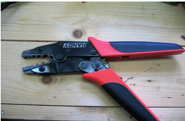
This is when you use the crimp tool. For RG8X it uses the second largest hex shaped hole in the crimp die.
