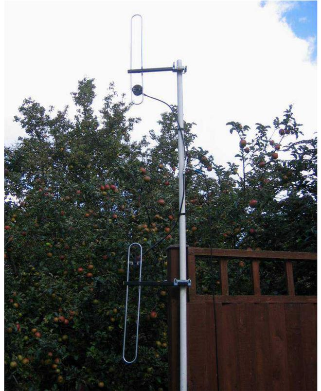
Based on a suggestion from John G8MNY, I mounted the lower Slim Jim upside down. The picture above shows them on the pole at ground level. I did a test with them mounted about 25 feet above ground and they performed about one S point better than the 2m Slim Jim was on 70cm. The SWR was low: varying from 1.2 to 1.4:1 from 430MHz to 440MHz. Maybe I’ll ask Quin G3WRR if he can model it for me.
