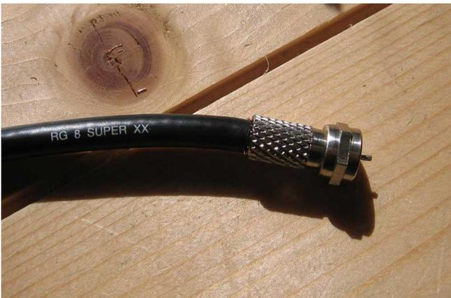
The inner of the RG8X is soldered to make it solid and avoid fraying.
