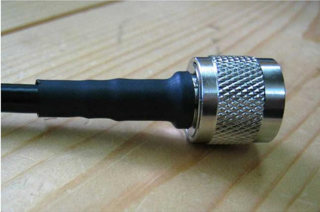
If the connector is destined for outdoor use I usually add a second sleeve that goes over the collar of the N connector with some silicon grease in between the two layers of heat shrink tubing.
