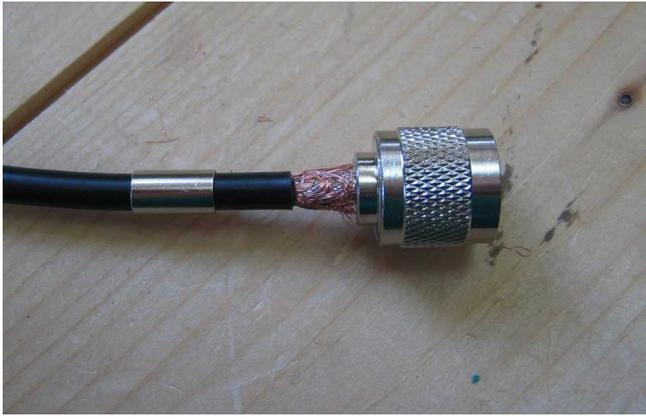
Push the cable assembly with centre pin into the N connector housing ensuring the braid stays on the outside.
