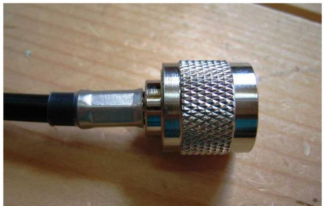
After applying heat, the sleeving shrinks to a tight fit around the crimp sleeve.
