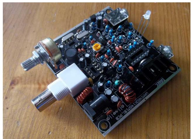
The bi-coloured LED (green for receive, red for transmit) I've left on its legs with a view (maybe) to housing it in a box - making removal easier.
