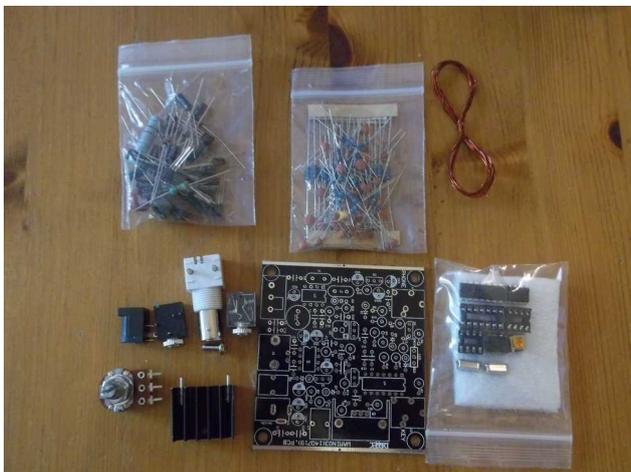
There is also an on-board oscillator to provide a side tone to monitor sent code via the 'phones; nice touch! All delivered for about £6. The circuit is a direct conversion receiver using a NE602 for the oscillator ( $\pm 7.023\text{MHz}$ ) and balanced mixer and a FET PA.
